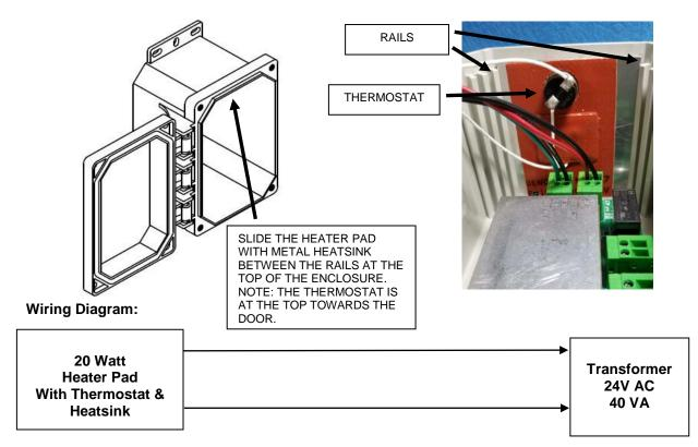
The heater kit comes complete with heater pad, thermostat, heatsink, and transformer:
